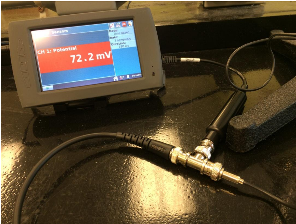
Figure A.2 BNC-T connection to the LabQuest unit
